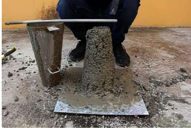
FIG SHOWS DETERMINATION OF SLUMP VALUE
