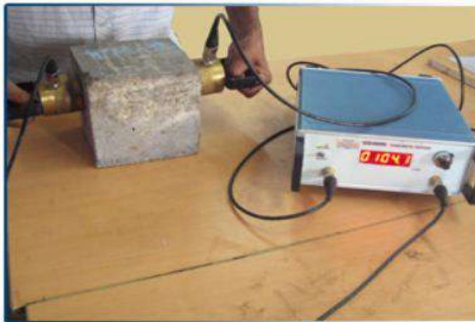
Figure 8 UPV test being conducted on a sample of concrete taken from a beam.
