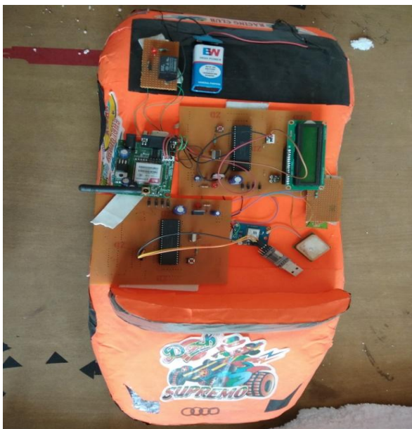
Fig.5: Hardware of tracking and controlling of theft car system on prototype car
