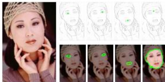
Fig (4.2): The fixations, indicated by the green circular dots on the different parts of the face, are shown overlaid on the inverse probabilistic edge map of the leftmost image. The segmentation corresponding to every fixation as given by the proposed algorithm is shown right below the edge map with the fixation.
