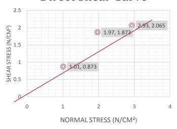
For untreated soil at 0%-Cohesion = 0.2 N/Sq. cm & angle of internal friction = 35.75 degree. AT 1%
