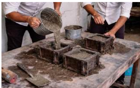
Figure 5.3: Pouring the Concrete into the Moulds
