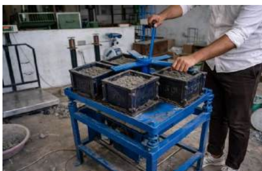
Figure 5.5: Compaction using Vibrator
