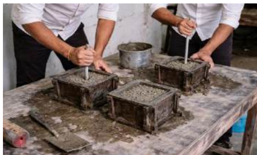
Figure 5.2: Preparation of Cube Moulds
