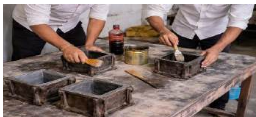
Figure 5.2: Preparation of Cube Moulds
