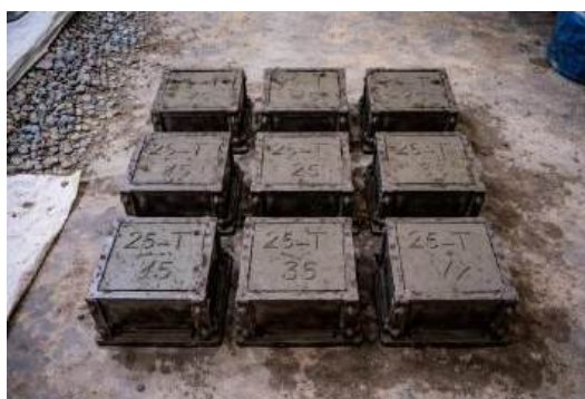
Figure 5.6: Giving Id's for cubes after compaction.
