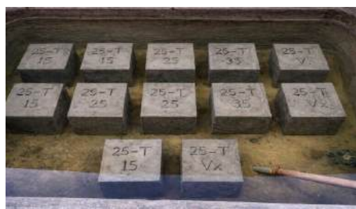
Figure 5.7: Curing of Concrete Cubes
