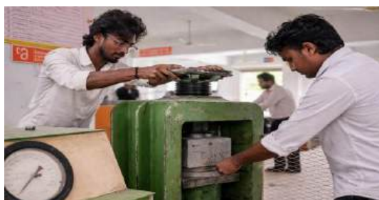
Figure 5.8: Conducting Compression Test on CTM
