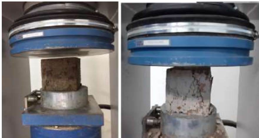
Figure 10 Samples during Compression test
