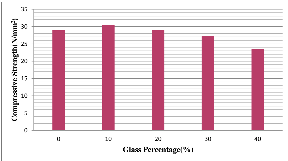
Figure 3: 28 days compressive strength vs percentage of glass replacement
