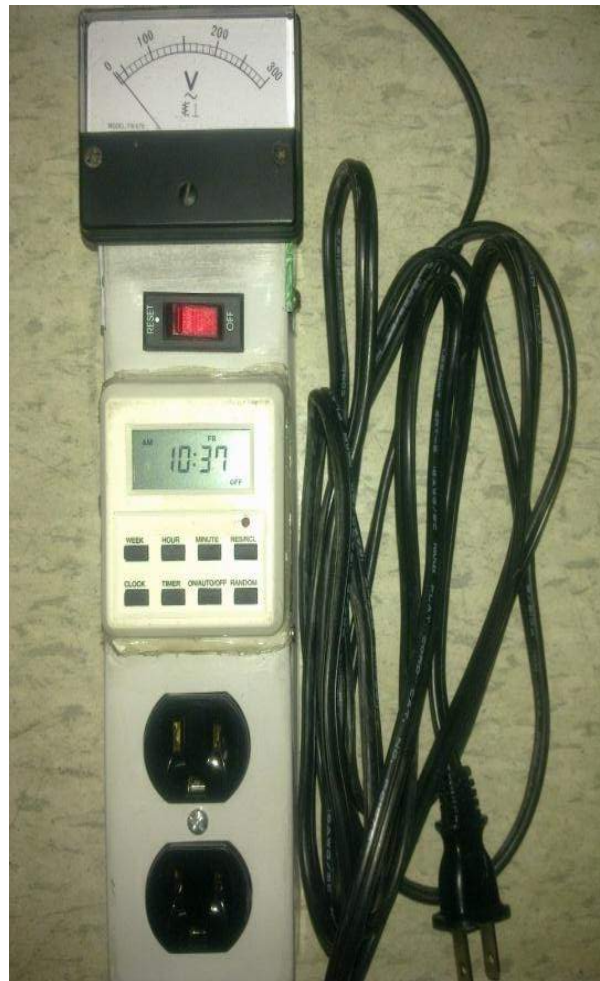
Figure 3 Actual Image of the Automatic Shut Off/On Extension Cord
