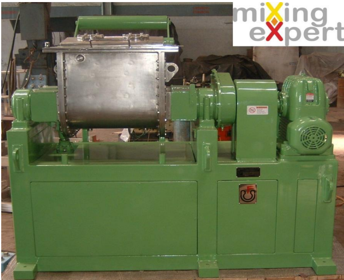
Figure No. 3: Sigma Mixer SM100 supplied by Unique Mixers and Furnaces Pvt.Ltd to ISRO Sriharikota.
