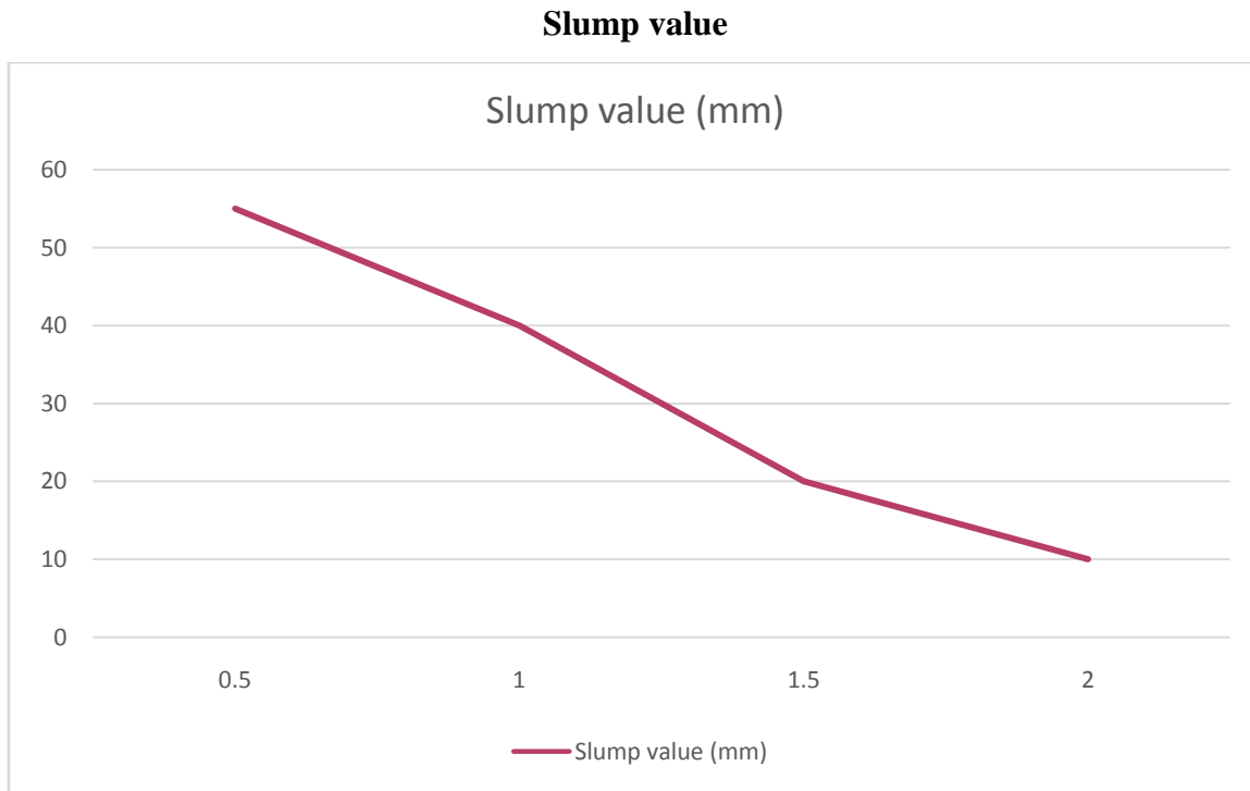
Fig -1: Slump values vs fiber volume fraction
