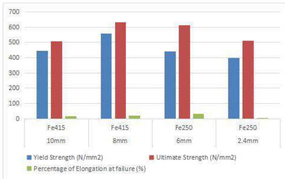
Fig 4: Yield strength, ultimate strength & % elongation of failure of wire mesh and different grades of steel
