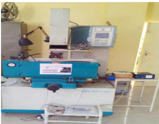
Figure 2. ZNC EDM machine with PMAEDG set up and Automated X axis
