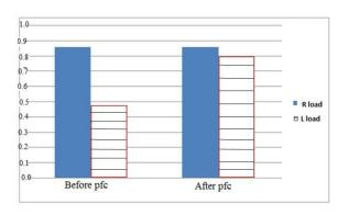
Shown estimation of power factor. Inductive load should be lagging nature and restive load unity nature. Analysis of before operating at inductive load poor power factor value 0.5-0.6.identified to signal automatically relay drive circuit on
