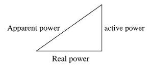
One of the major causes of this poor power factor due to inductive loads which causes a phase difference in voltage and current. Thus an improved power factor leads to reduction in VA demand and hence the user can conserve billing if improvements in power factor improve system efficiency. in
